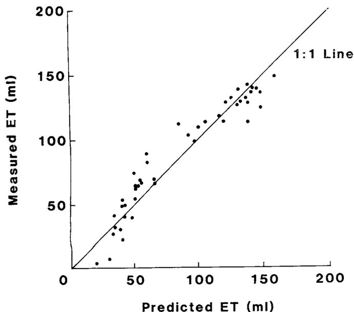
Fig. 1. Measured evapotranspiration (ET) values versus ET values predicted from Eq [2].
