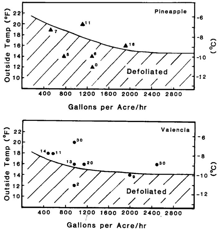
Fig. 7. Protection level provided for (a) Pineapple or (b) Valencia oranges by microsprinkler irrigation. Volume applied is compared with outside temperature in a non-irrigated adjacent block. The number by each data point indicates the damage rating. Trees with a rating of 9 or below were defoliated.
