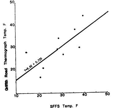
Fig. 4. Line of best fit giving a correlation coefficient of 0.82 for 9 observations taken at 8:00 p.m., 1:00 a.m. and 6:00 a.m. on January 10-11, 11-12 and 12-13, 1981, Griffith Road thermograph station. Note scatter of observation points around line of best fit.
