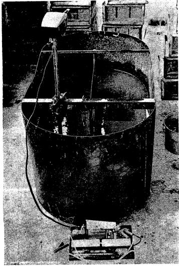
Fig. 2. A muscadine grape continuous flow density separator.
