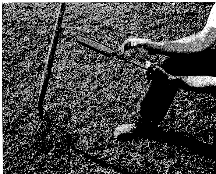
Fig. 1. Manure fork with attached scale used for determining tensile strength of the sod.
