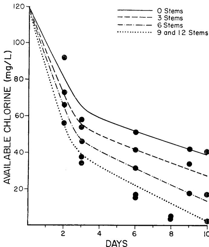
Fig. 3. Influence of the number of carnation stems on available chlorine in sodium dichloroisocyanurate (DICA) and sucrose (SU) after 10 days. (Curved lines fitted by eye.)
