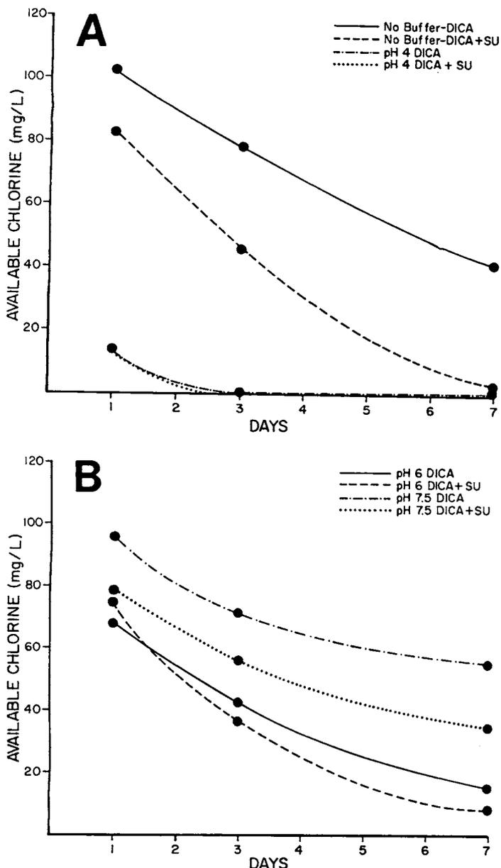
Fig. 1. Influence of buffering and sucrose (SU) on available chlorine in sodium dichloroisocyanurate (DICA) solutions after 7 days. (Curved lines were fitted by eye. Buffer, sucrose main effect and buffer x sucrose interaction significant at the 5% level for day 1, 3 and 7.
