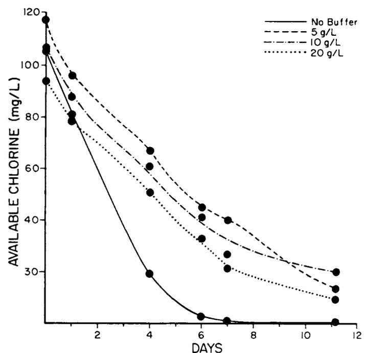
Fig. 2. Influence of citrate-phosphate buffer concentrations on available chlorine in sodium dichloroisocyanurate and sucrose solutions after 11 days. (Curved lines fitted by eye. Means of each buffer concentration are significantly different from control (no buffer); but, not significantly different from each other at day 4, 6, 7, and 11. There are no significant differences at day 1.)
