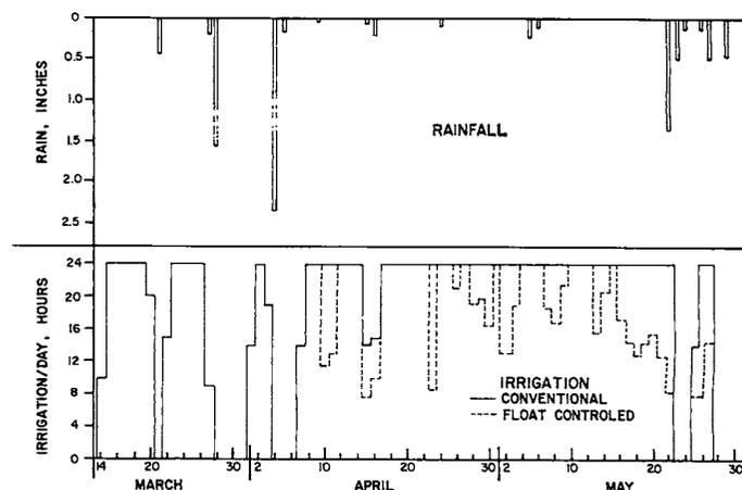
Fig. 4. Rainfall and irrigation hours of operation for the float-controlled and conventionally-managed seepage irrigation systems at the Yelvington Research Farm in 1984.
