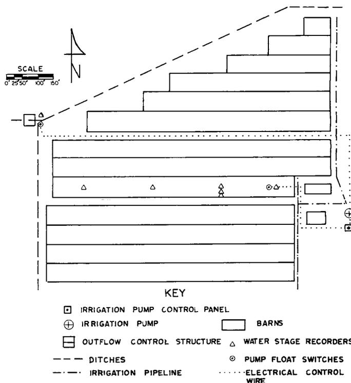
Fig. 1. Float-controlled irrigation system layout at the Hastings Agricultural Research and Education Center main laboratory farm.
