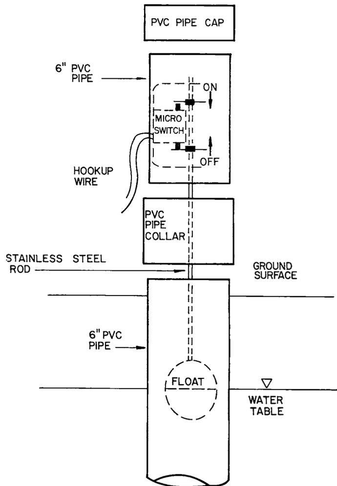
Fig. 2. The pump control float switch we designed to turn the irrigation pumping system on and off in response to water table elevations.
