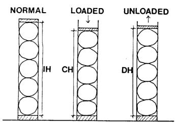
Fig. 2. Grierson CreepTester methodology. IH = initial height; CH = compressed height; DH = decompressed height. Permanent deformation = (IH - DH) x 100/IH. Percentage elasticity = ((DH - DH) x 100/IH. Percentage elasticity)CH)/ (IH - CH)) x 100. After Rivero, et al. (12).
