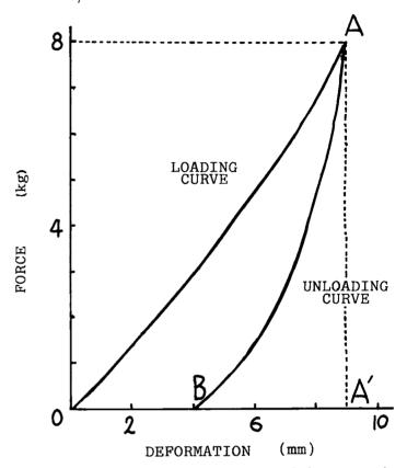
Fig. 1. Force-deformation curve of 'Marsh' grapefruit to compression by loading to 8 kgf (78.5 N) and then unloading to 0 kgf as a speed of 5mm/min. Stiffness:AA'/OA'. Initial deformation: OA'. Percentage of permanent deformation: OB/OA' x 100.
