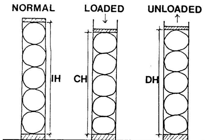
Fig. 2. Grierson CreepTester methodology. IH = initial height; CH = compressed height; DH = decompressed height. Permanent deformation =  $(IH - DH) \times 100 / IH$ . Percentage elasticity =  $((DH - CH) / (IH - CH)) \times 100$ . After Rivero, et al. (12).
