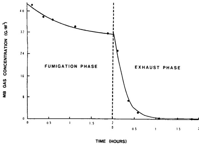
Fig. 2. Gas concentration readings taken during a typical methyl bromide fumigation of a semi-trailer load of grapefruit in a 266-m<sup>3</sup> chamber. Dosage applied: 40 g/m<sup>3</sup>. Each point on the curve represents the mean reading for 12 sampling points within the chamber.
