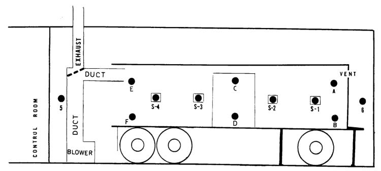
Fig. 1. Location of gas-sampling leads in the USDA 266-m<sup>3</sup> fumigation chamber, Miami, FL.
