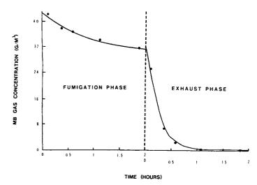
Fig. 2. Gas concentration readings taken during a typical methyl bromide fumigation of a semi-trailer load of grapefruit in a 266-m<sup>3</sup> chamber. Dosage applied: 40 g/m<sup>3</sup>. Each point on the curve represents the mean reading for 12 sampling points. within the chamber.
