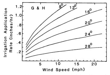
Fig. 5. Sprinkler application rates required for cold protection to different levels as determined by the Gerber and Harrison model.
