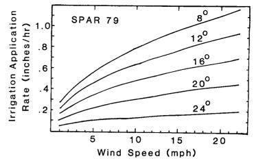
Fig. 6. Sprinkler application rates required for cold protection to different levels as determined by the SPAR 79 model.
