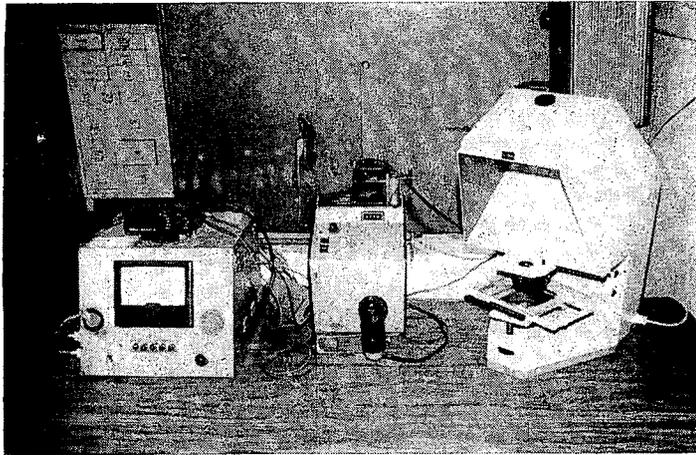
Fig. 1. Spectral densitometer set up.
