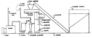
Fig. 2. Downdraft gasifier system.
