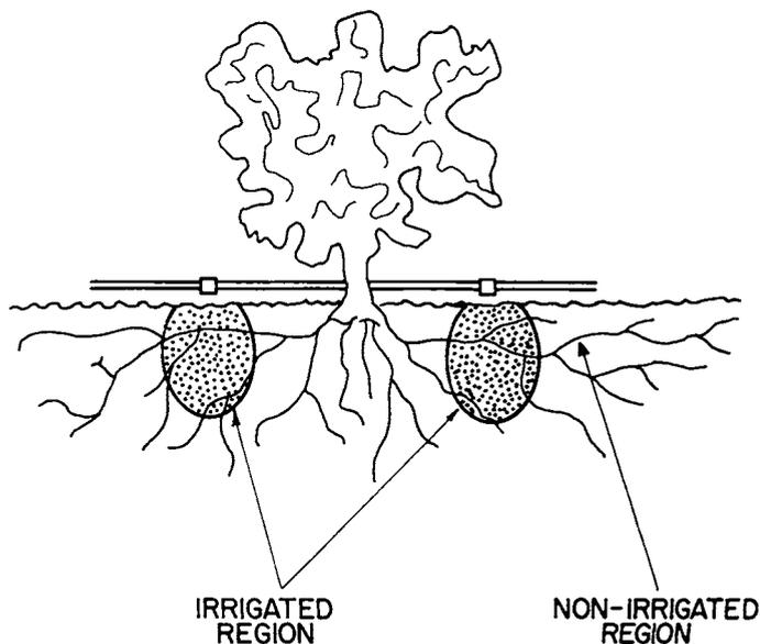
Fig. 1. Soil moisture regions under a trickle irrigated crop.
