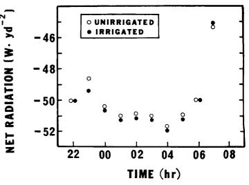
Fig. 4. Net radiation 32 in above the soil surface 2-year-old 'Hamlin' orange trees during a radiative freeze on 11-12 Jan. 1987. Points are means of 4 values for irrigated and unirrigated treatments.
