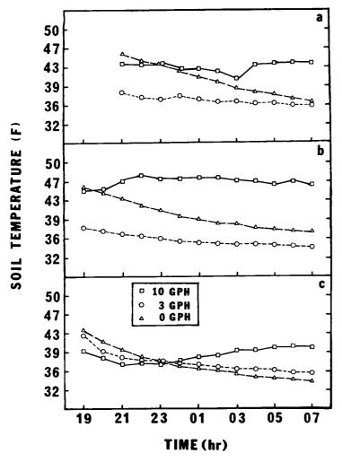
Fig. 5. Soil temperature measured 0.5 in below the surface and next to trunks of 2-year-old 'Hamlin' orange trees during freezes on 25-26 Dec. 1985 (a), 26-27 Dec. 1985 (b), and 27-28 Jan. 1986 (c). Points are single values for the unirrigated (0 GPH), 3 gal per hr (3 GPH) and 10 gal per hr (10 GPH) treatments.
