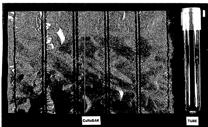
Fig. 1. Falcon CultuSAK™ (CK) culture system consisting of five cells each having the volume of a standard 150 x 25 mm glass culture tube. Scale bar = 1.0 cm.
