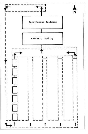
Fig. 2. Diagram of a proposed mobile strawberry production system, showing the position of the mobile units in the field and the direction of their movement, first through a harvest/cooling facility, and then through a spray/steam sterilization facility.
