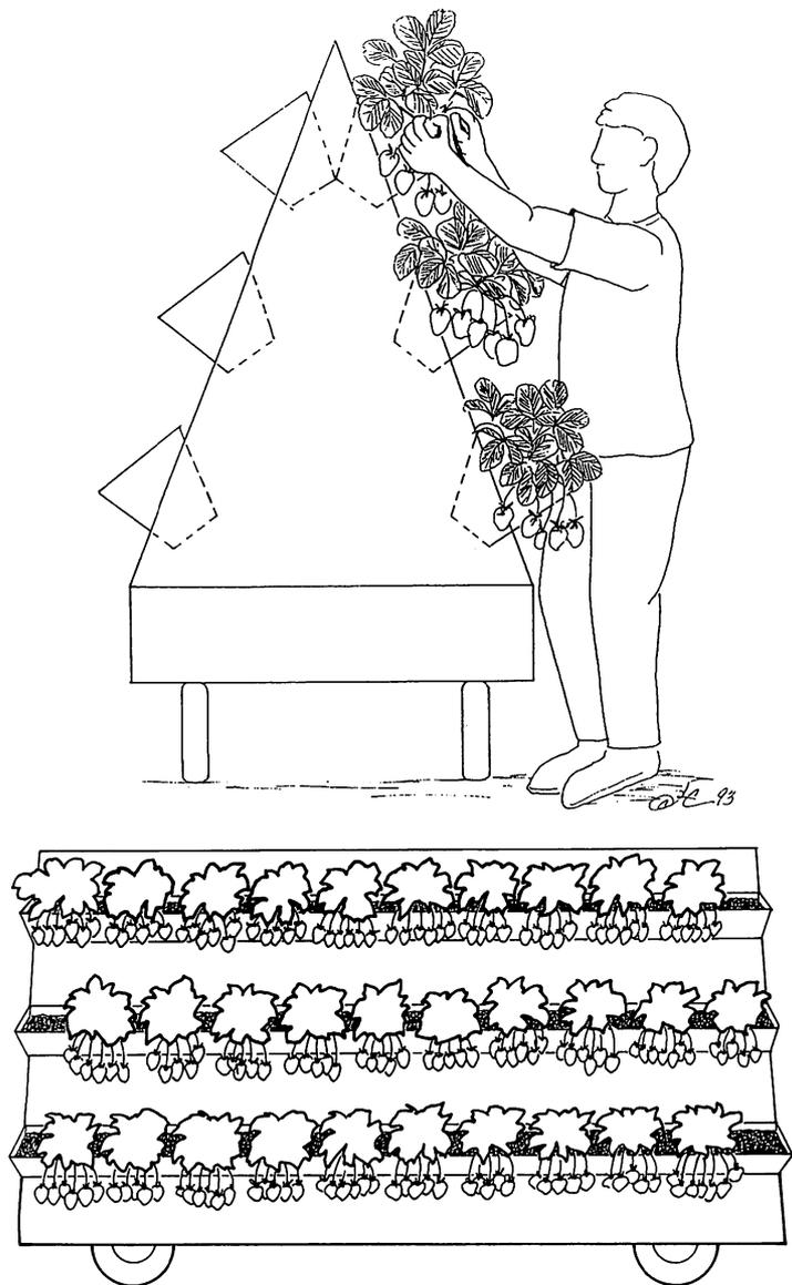
Fig. 1. End and side view of a proposed mobile strawberry growing unit.
