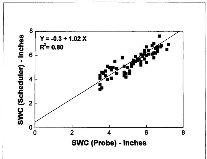
Figure 6. Predicted (scheduler) soil water content verses measured (neutron probe), 1994.
