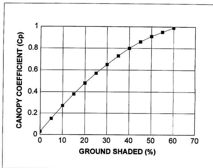
Figure 2. Canopy coefficient as a function of ground shaded at solar noon during mid-season.
