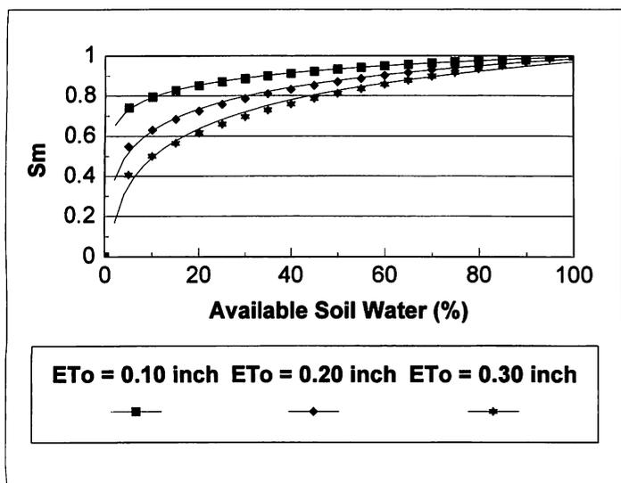
Figure 3. Soil moisture availability as a function of soil water content and  $ET$ .
