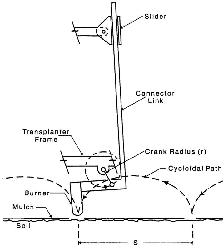
Figure 1. Burner on a slider crank mechanism.
