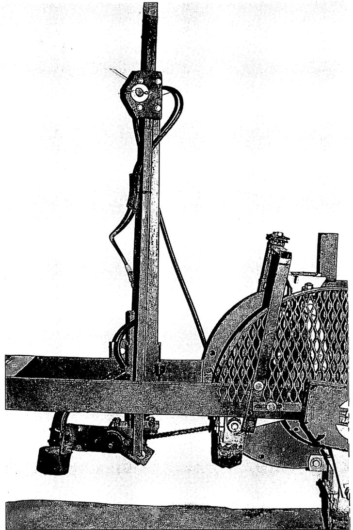
Figure 2. Transplanter with cycloidal hole burner.
