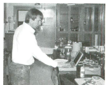
Mr. Craig Davis, Associate Research Scientist, measuring fruit internal temperatures with a data-logger.
