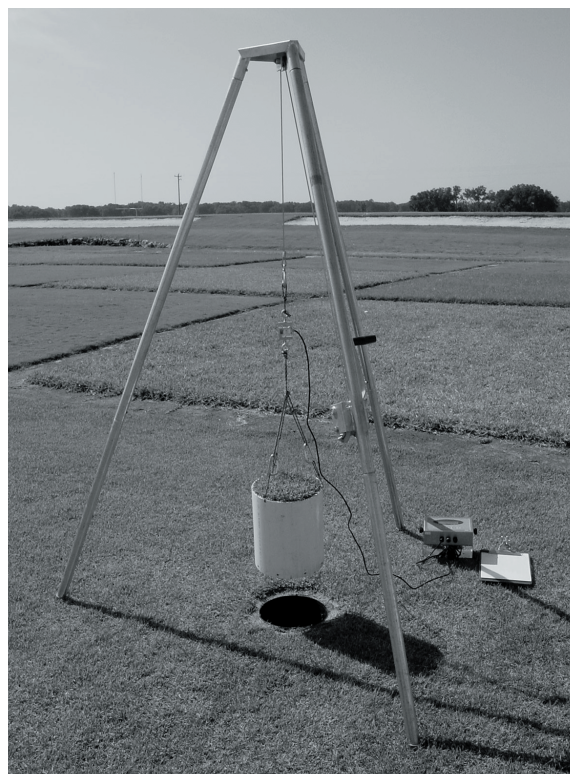
Fig. 2. Photograph of tripod placement, hoist, load cell, harness, lysimeter, and output display.
