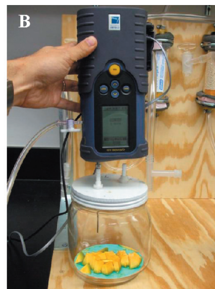
Fig. 3. (A) Apparatus constructed to improve the accuracy of the electronic nose, based on the apparatus developed by M.O. Balaban and Luis Martinez (Martinez, 2007). Design used with permission. (B) Detail of headspace sample draw.
