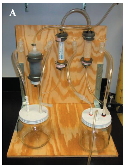
Fig. 3. (A) Apparatus constructed to improve the accuracy of the electronic nose, based on the apparatus developed by M.O. Balaban and Luis Martinez (Martinez, 2007). Design used with permission. (B) Detail of headspace sample draw.
