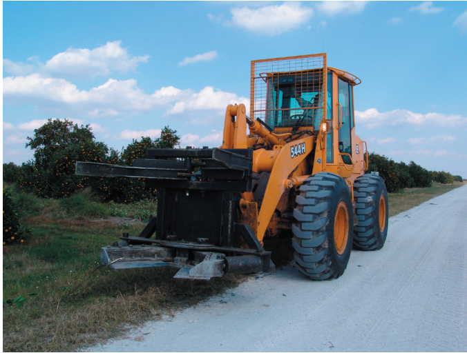
Fig.1. Front-end loader used in clipping citrus trees with tree shear attachment.
