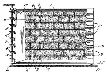
Fig. 2. Lateral brusher. Fruit travels along brush groves from left to right. Often sloped downhill to encourage fruit movement (From US Patent 1,417,266).
