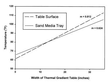
Figure 3. Temperatures measured on the thermal gradient table surface and in the sand media tray.
