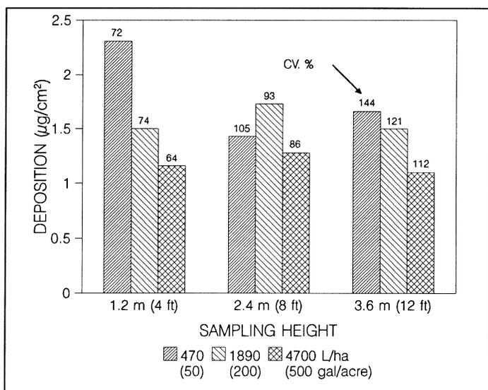
Figure 3. Mean and CV of deposition at different sample heights.
