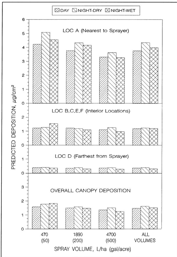
Figure 5. Predicted deposition for day and night applications at different radial locations.
