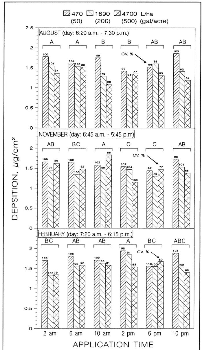
Figure 2. Mean and CV of deposition for different application times and spray volumes. Average deposits of the 6 application times (within each month) are separated by Fisher's protected LSD at the 5% level.
