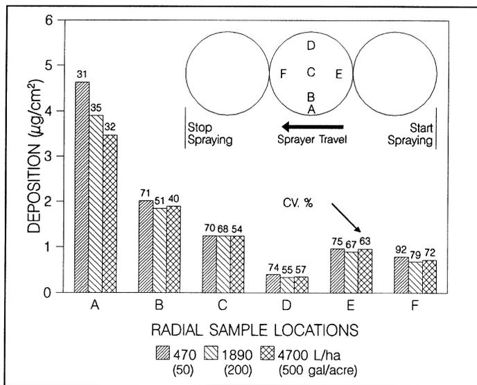
Figure 1. Schematic view of the sprayed trees and radial sample locations. Mean and CV of deposition for different volumes and sample locations.
