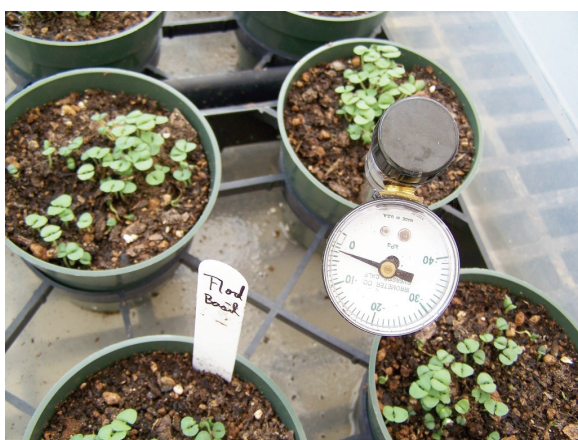
Fig. 1. Miniature tensiometer installed in a 4-inch pot as part of an irrigation study with organic herbs.
