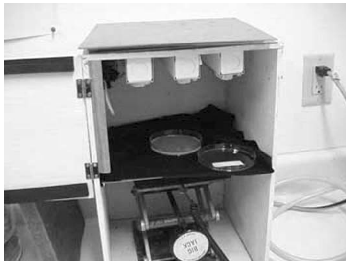
Fig. 1. UV-C germicidal light used in the experiments.
