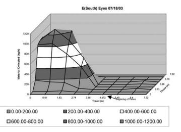
Fig. 4. Typical response start-up pattern and distribution for standardized open-field spreader tests (SI conversions: 1m = 3.28 ft, 1 kg/ha = 0.89 lb/A).
