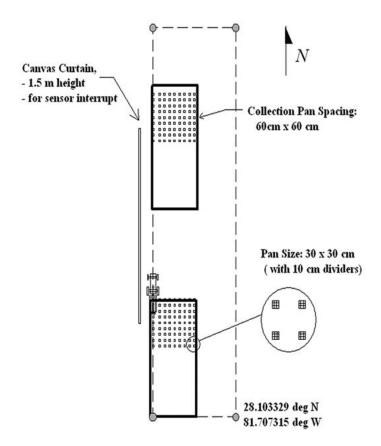
Fig. 1. Test area for dynamic response tests of granular fertilizer applications.
