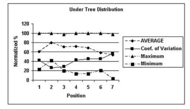
Fig. 5. Under-tree tray collection of dry fertilizer distribution presented as normalized values representing ratio of mass of fertilizer collected at  $i^{th}$  position divided by maximum amount of material collected at any position for each test. Trays positioned on 2 ft (51 cm) centers with position <u>4</u> at centerline of tree row.
