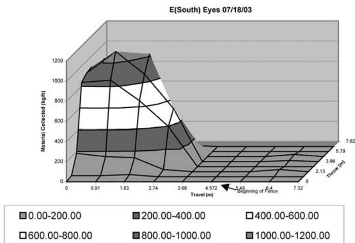
Fig. 4. Typical response start-up pattern and distribution for standardized open-field spreader tests (SI conversions: 1m = 3.28 ft, 1 kg/ha = 0.89 lb/A).
