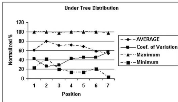
Fig. 5. Under-tree tray collection of dry fertilizer distribution presented as normalized values representing ratio of mass of fertilizer collected at  $i^{th}$  position divided by maximum amount of material collected at any position for each test. Trays positioned on 2 ft (51 cm) centers with position 4 at centerline of tree row.
