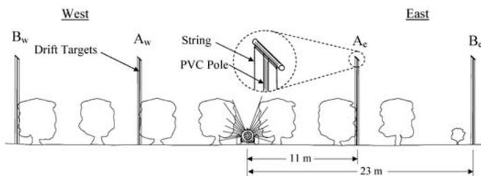
Fig. 1. Schematic view of spray application and drift target locations
