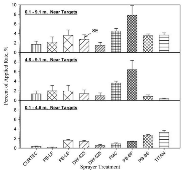
Fig. 6. Comparative drift deposits of the sprayers at and above canopy levels.
