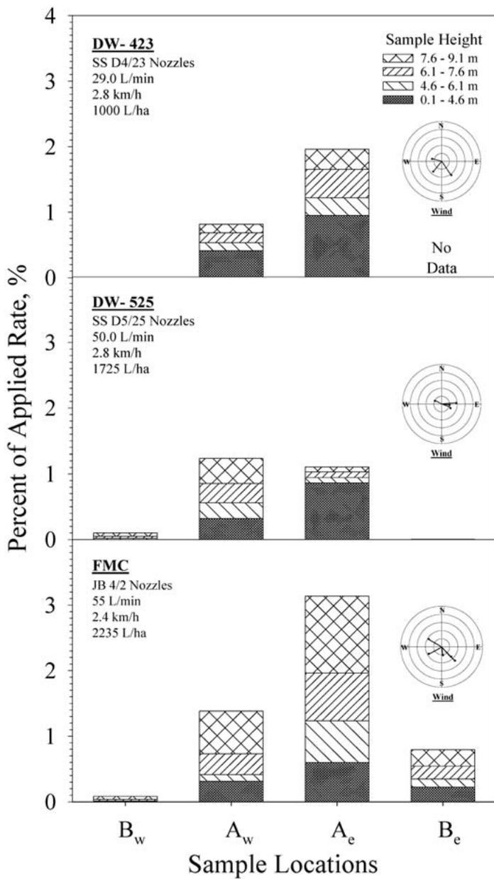
Fig. 3. Spray drift deposits of the Durand-Wayland and FMC sprayers.
