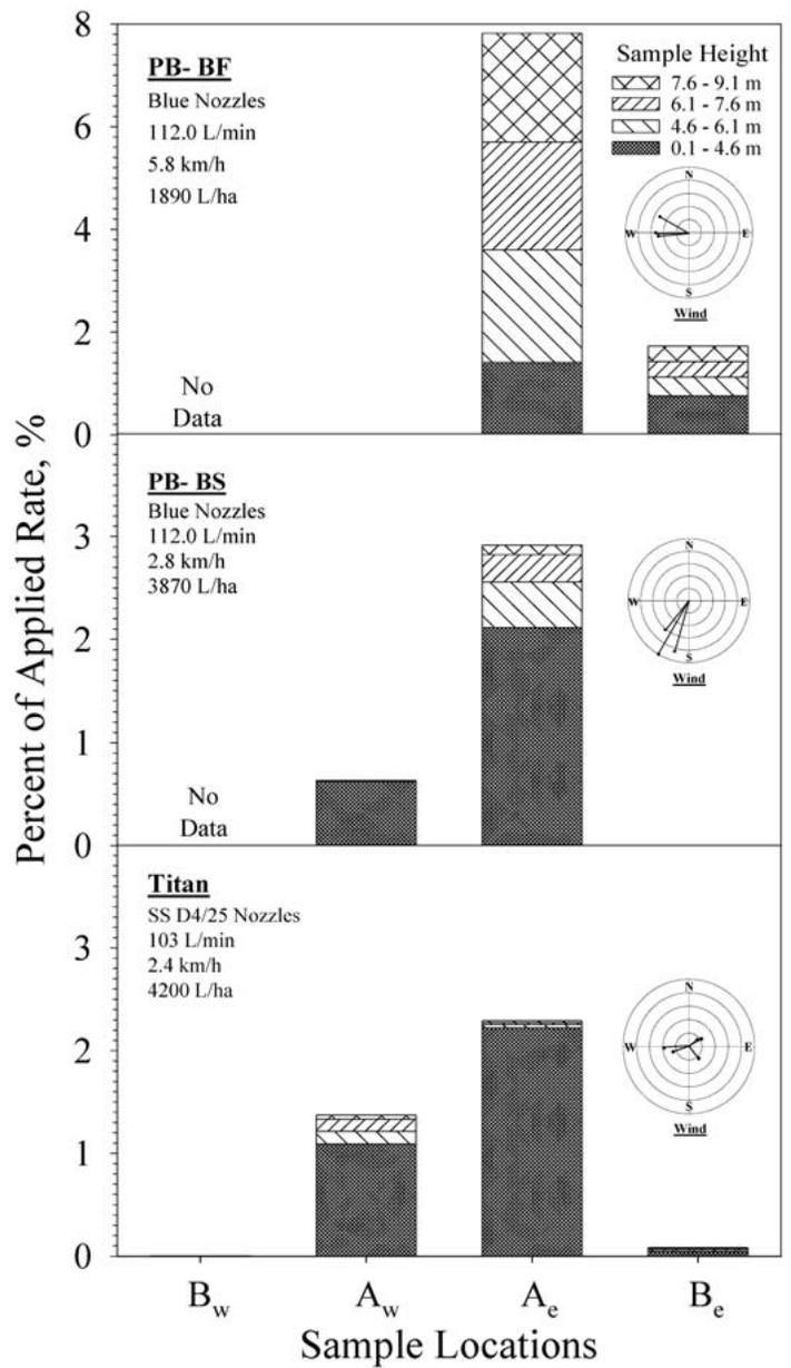
Fig. 4. Spray drift deposits of the high-volume Power-Blast and Titan sprayers.
