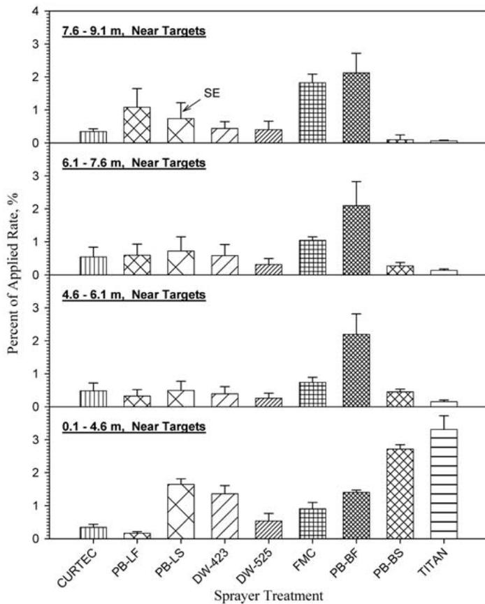
Fig. 5. Comparative drift deposits of the sprayers at different sampling heights.
