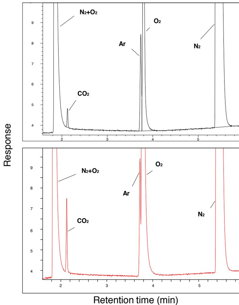
Fig. 2. The separation as seen on the TCD. The chromatogram on top shows 0.1% CO<sub>2</sub>, 1% Ar, 5% O<sub>2</sub> and 97.9% N<sub>2</sub>. The chromatogram on the bottom shows 0.4% CO<sub>2</sub>, 1% Ar, 17% O<sub>2</sub> and 81.6% N<sub>2</sub>.
