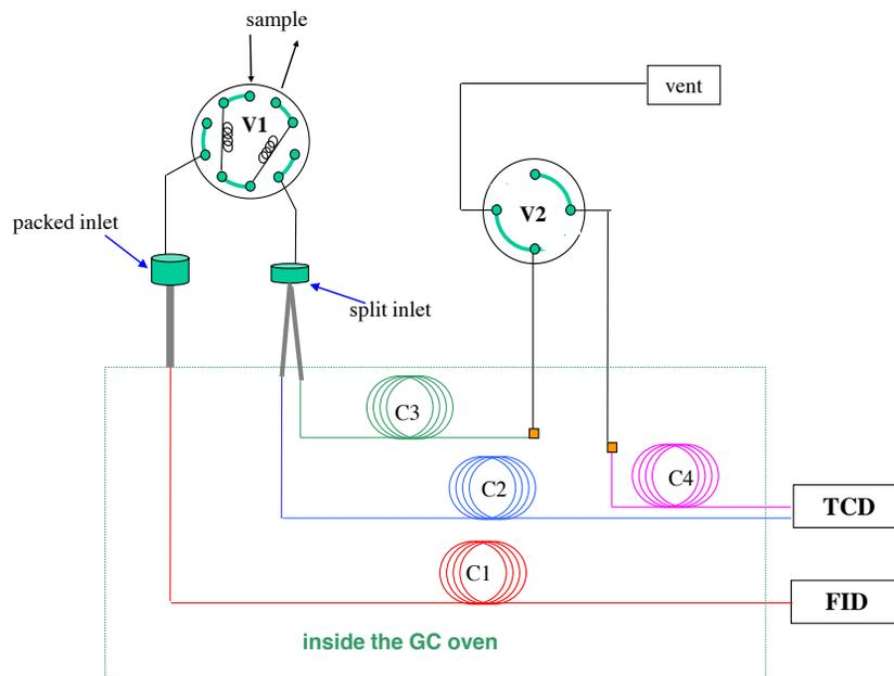
Fig. 1. GC configuration and operation scheme. C1–C4: columns; V1 and V2: valves. See Tables 1 and 2 for model and technical parameters of the major components. TCD: thermal conductivity detector. FID: flame ionization detector.
