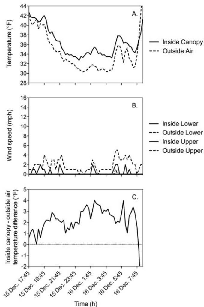
Fig 3. (A) Inside canopy and outside air temperatures, (B) wind velocities inside and outside grove, and (C) temperature difference between inside citrus tree canopy and outside grove air temperature from 15 Dec. 17:45 to 16 Dec. 08:30HR.
