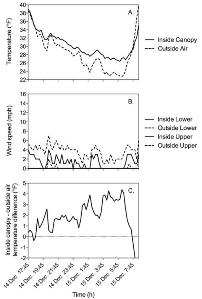
Fig 2. (A) Inside canopy and outside air temperatures, (B) wind velocities inside and outside grove, and (C) temperature difference between inside citrus tree canopy and outside grove air temperature from 14 Dec. 17:45 to 15 Dec. 08:30 HR.
