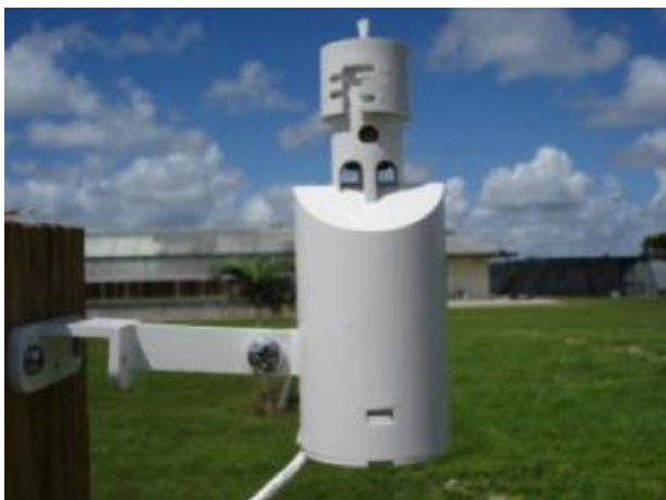
Fig. 5. Example of rain sensor. Credit: Nicole A. Dobbs, UF/IFAS.
