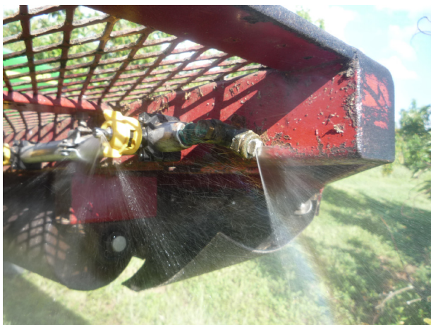
Fig. 2. Herbicide boom with Quick Turbo FloodJet® nozzles spaced 20 inches apart and one flat-fan nozzle at the end of the boom.
