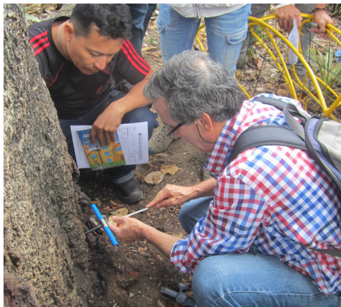
Fig. 1. León Morales assessing tree decay using an increment borer
