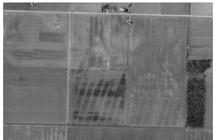
Fig. 18. Detecting old drainage lines by using UAV imagery.
