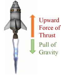
$$F_{Thrust} - F_{gravity} = m \cdot a$$
