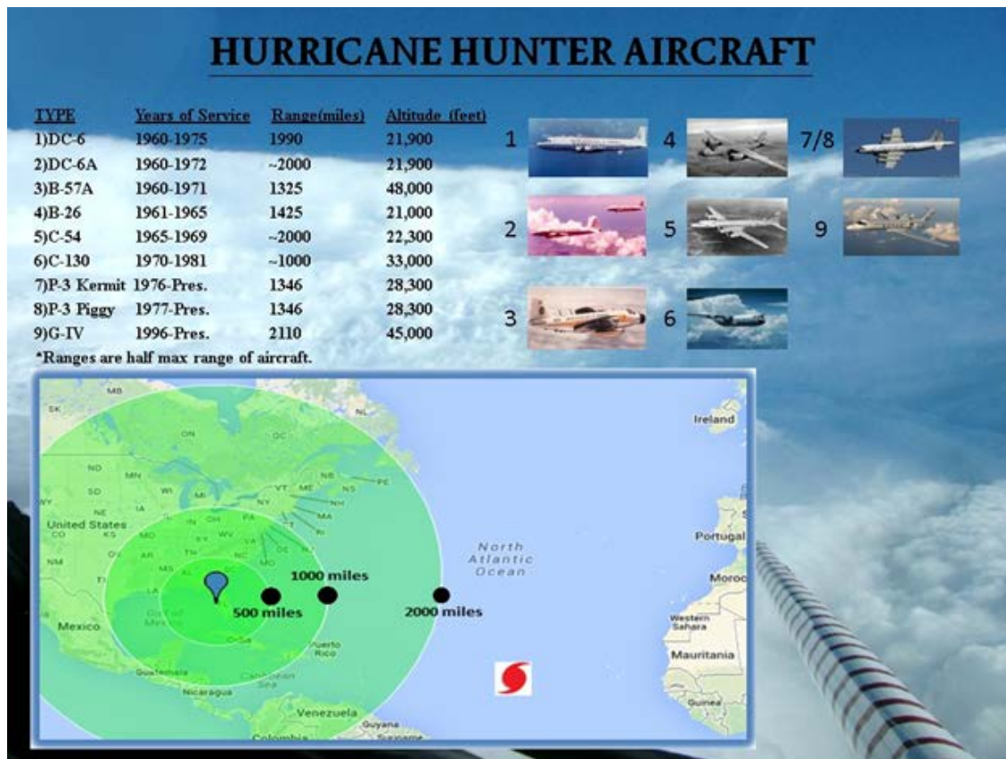
Figure 5. History of the AOC’s Hurricane Hunter Aircraft Dating Back to 1960. In this figure are the years the aircraft flew research and recon missions, along with their respective maximum altitudes and ranges. Note that these ranges are half of the maximum range for the aircraft, an depict how far out the plane can fly before having to return back to base. The background image is of an eyewall penetration intoHurricane Katrina (2005). (Figure arranged by Randall Hergert, University of South Florida).
