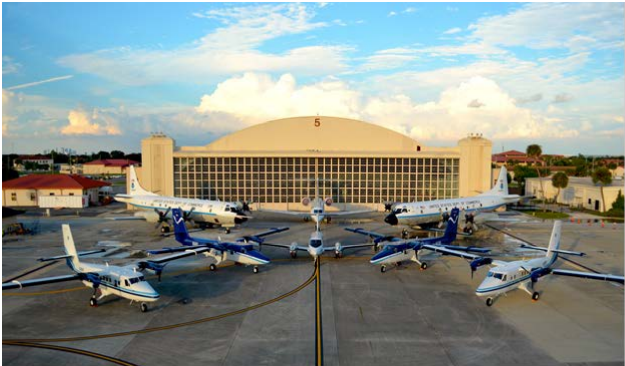
Figure 4. NOAA's Aircraft Operations Center Fleet. The NOAA G-IV is at the back middle, the two WP-3D Orion planes are at the back right and left, the King Air is at the front middle, the Turbo (Jet Prop) Commanders are at the front, and the Twin Otters are the blue planes (second from front) (Courtesy of NOAA AOC)
