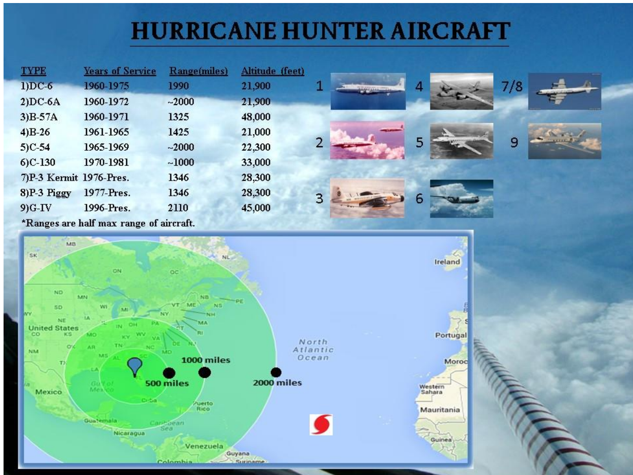
Figure 5: History of the AOC’s Hurricane Hunter Aircraft Dating Back to 1960. In this figure are the years the aircraft flew research and recon missions, along with their respective maximum altitudes and ranges. Note that these ranges are half of what the maximum range for the aircraft is. These ranges more accurately depict how far out the plane can fly before having to return back to base. The background image is of an eyewall penetration into Hurricane Katrina (2005). (Figure arranged by Randall Hergert, University of South Florida)
