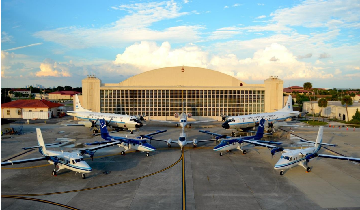
Figure 4: NOAA's Aircraft Operations Center Fleet. The NOAA G-IV is at the back middle, the two WP-3D Orion planes are at the back right and left, the King Air is at the front middle, the Turbo (Jet Prop) Commanders are at the front, and the Twin Otters are the blue planes (second from front).
