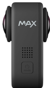
Figure 2: Side view of GoPro showing two lenses/ https://gopro.com/
