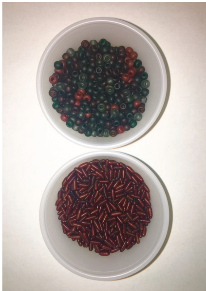
Fig. 1. A set of 1,000 live house fly puparia and an equal volume (33 cm 3 ) of the acrylic beads used in the assays to illustrate the general appearance of the bead decoys.
