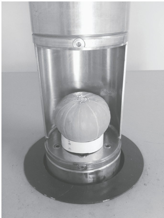
Fig. 2. Positioning of an Exallomochlus hispidus mealybug-infested squash fruit in the cavity of the \gamma -irradiator.
