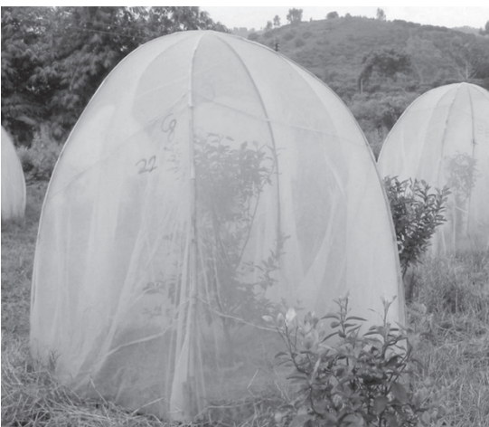
Fig. 2. Mesh cages used in the field experiment. Each cage contained one small (1.3 m tall) 4-yr-old Citrus reticulata tree. Thirty Diaphorina citri adults (1:1 sex ratio) together with various numbers of sachets of Neoseiulus cucumeris were released into each cage and changes in the D. citri population density over the subsequent 3 months were determined.
