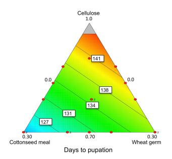
**Fig. 3.** Predicted 3-dimensional surface response plot of development for larval *D. abbreviatus* reared on diets with varying proportions of 2 major diet components (cottonseed meal and wheat germ) and a non-nutritive filler (cellulose). Values on plot are original scale.
