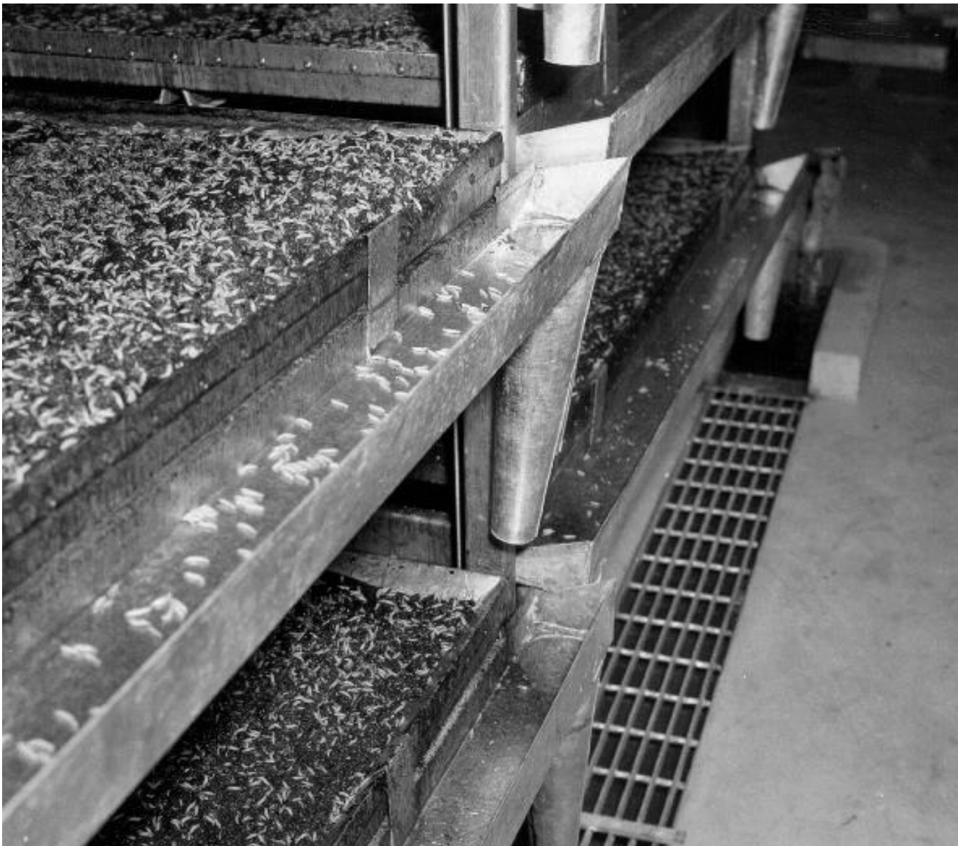
Fig. 13. Screwworm rearing vats. After 30 hours in the starting chamber the larvae were transferred to vats on the main floor. Diet was similar to the starting medium except that whole bovine blood was substituted for plasma. After 4 days larvae reached the size shown, migrated from the vat, and were directed to the water conveyor beneath the grate. (USDA)
