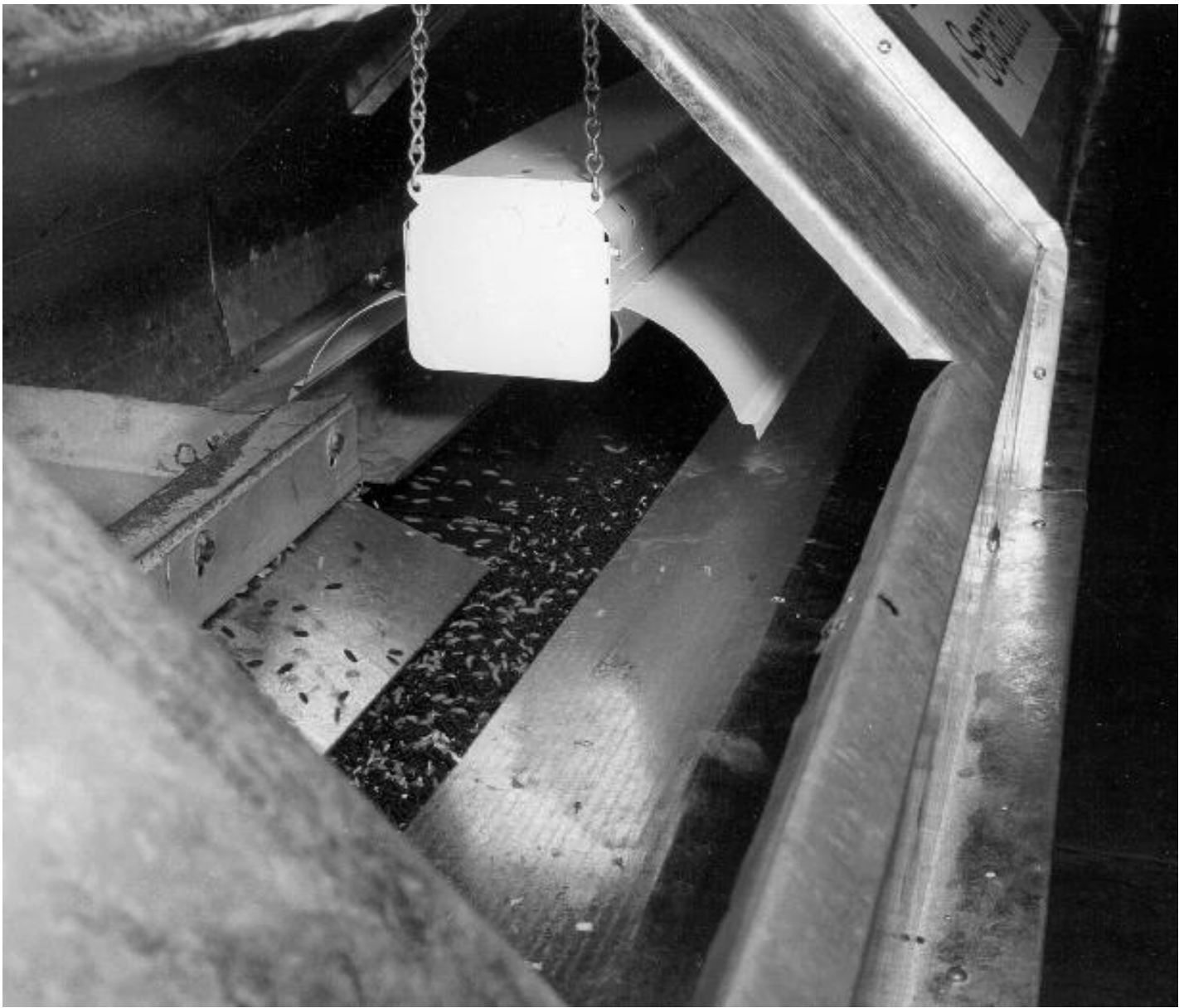
Fig. 15. Larva-pupa separator. The mixture of larvae and pupae was transported to a slowly moving endless belt. The negatively phototropic larvae crawled to the sides and dropped into containers for recycling in the pupation chamber. Pupae, remaining on the belt, were collected at the opposite end for storage. (USDA)
