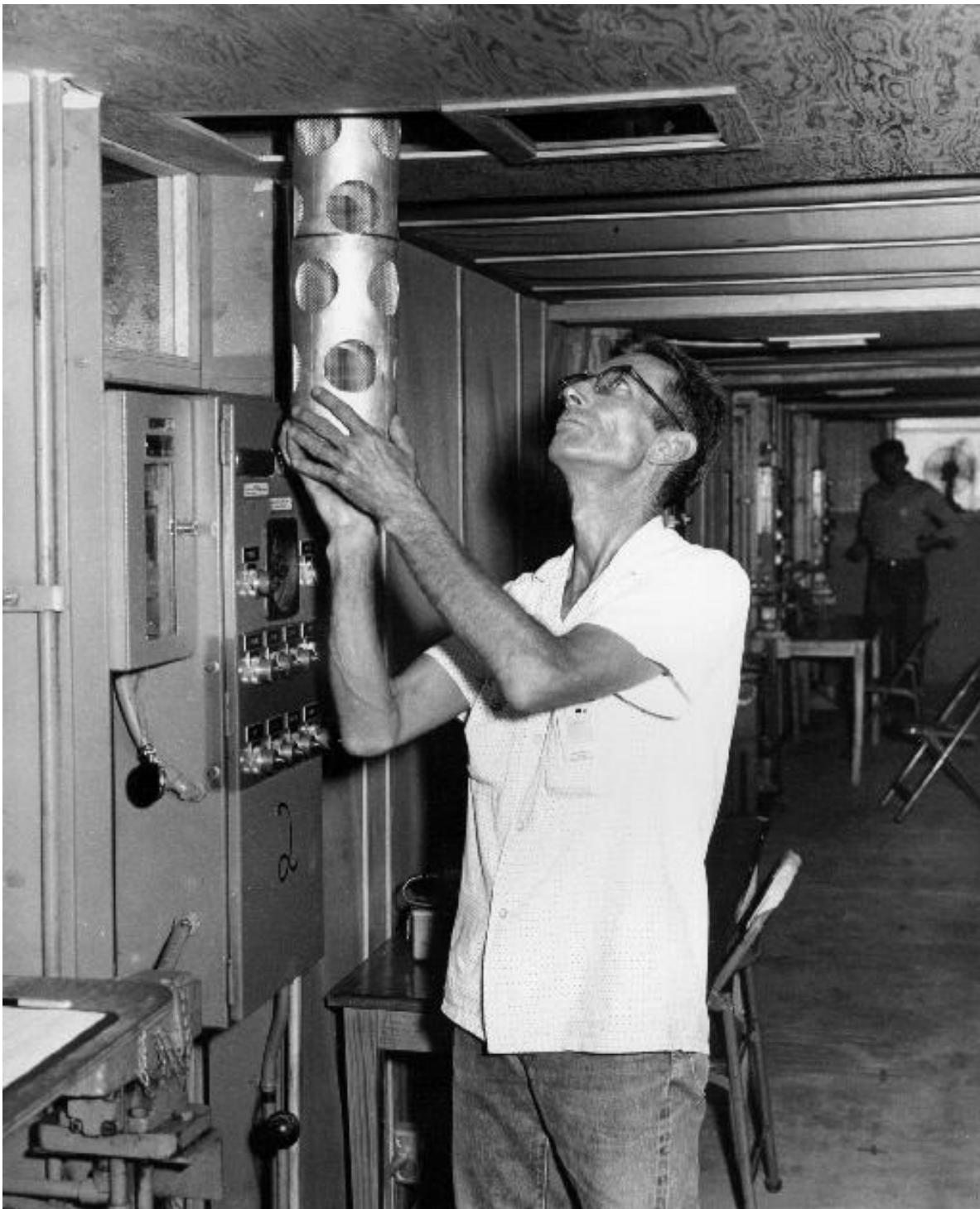
Fig. 17. Positioning irradiation canister on carrier, which inserted it into the irradiation chamber and automatically removed it at the scheduled time for transfer to the packaging area. (USDA)
