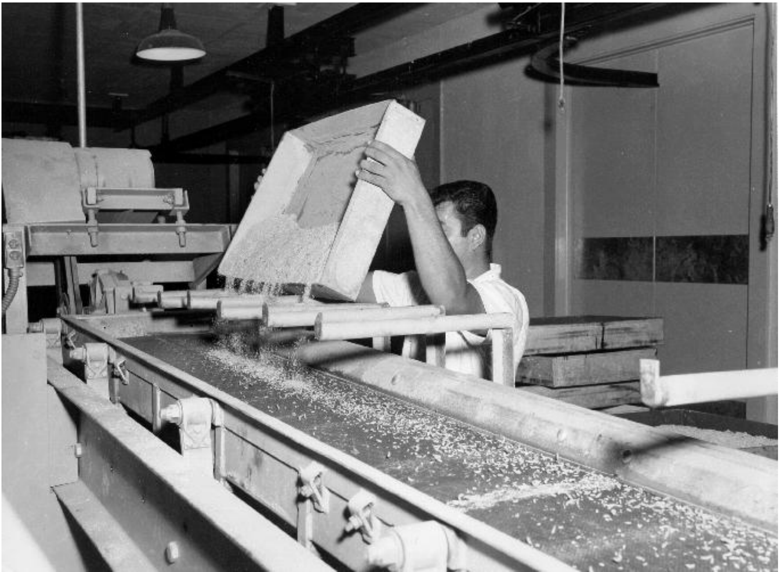
Fig. 14. Sawdust separator. Larvae were collected at the larva-water separator (not shown) and placed in pupation trays containing sawdust; 16 hours later the sawdust was removed from the mixture of larvae and pupae to permit separation of the life stages. (USDA)
