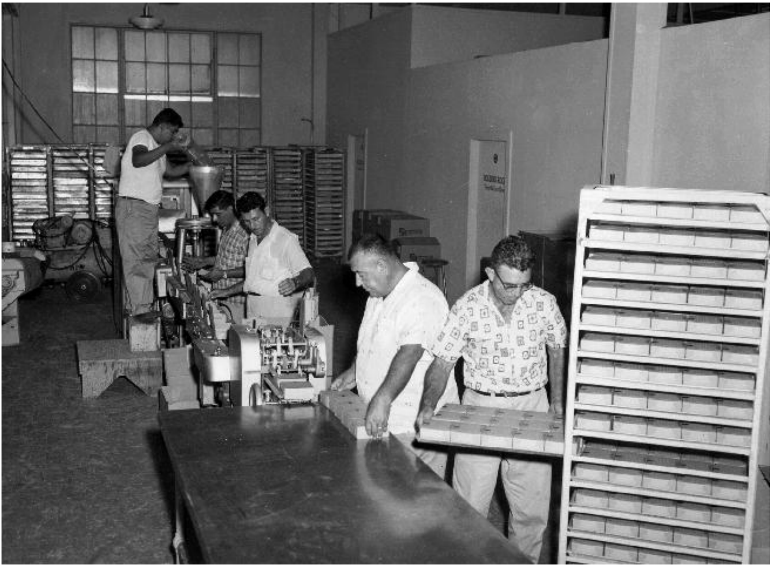
Fig. 19. Packaging line. Operator on stool emptied the irradiated screwworm pupae into an automatic filler which dispensed the pupae into the release cartons. Cartons were formed and closed mechanically at the rate of 50 per minute. (USDA)
