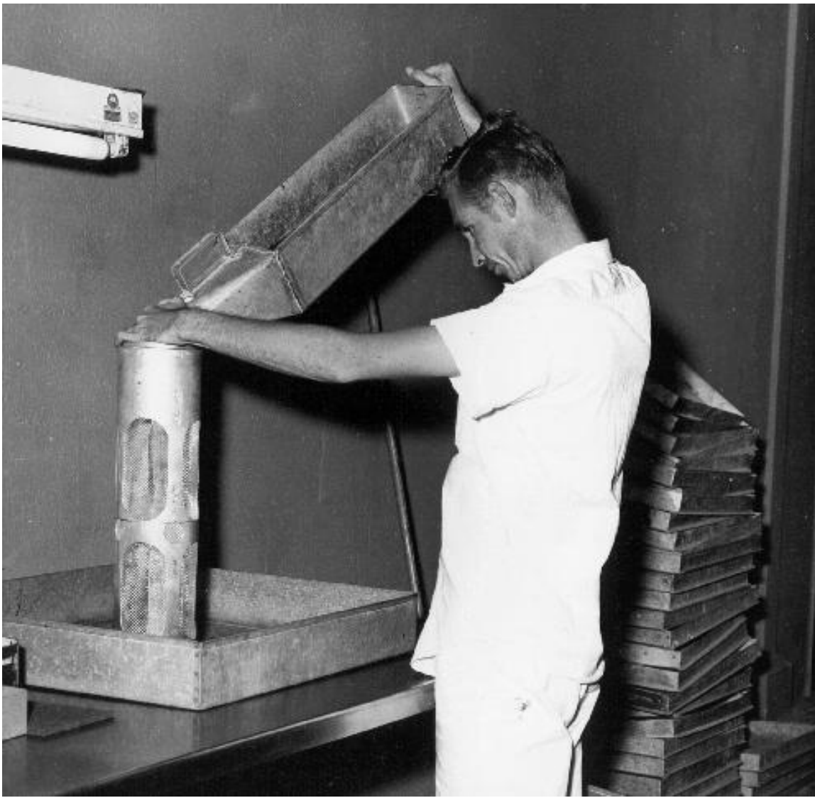
Fig. 16. Irradiation canister being loaded with 2 liters of pupae (18,000). Pupae received 8000r \pm 10\% at 5 1/2 days of age. (USDA)
