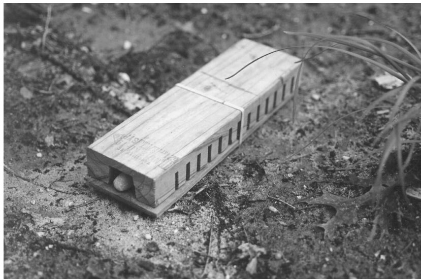
Figure 2. Completed trap, with a bottom plate.
