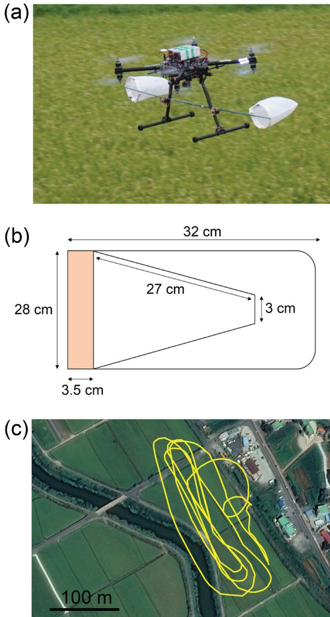
**Fig. 1.** Rotary-wing unmanned aerial vehicle equipped with remote-controlled insect net openings (a). Layout of double-layered insect net designed to prevent loss of insect samples during aerial sampling (b). Representative flight path of unmanned aerial vehicle for aerial sampling over rice field (c).
